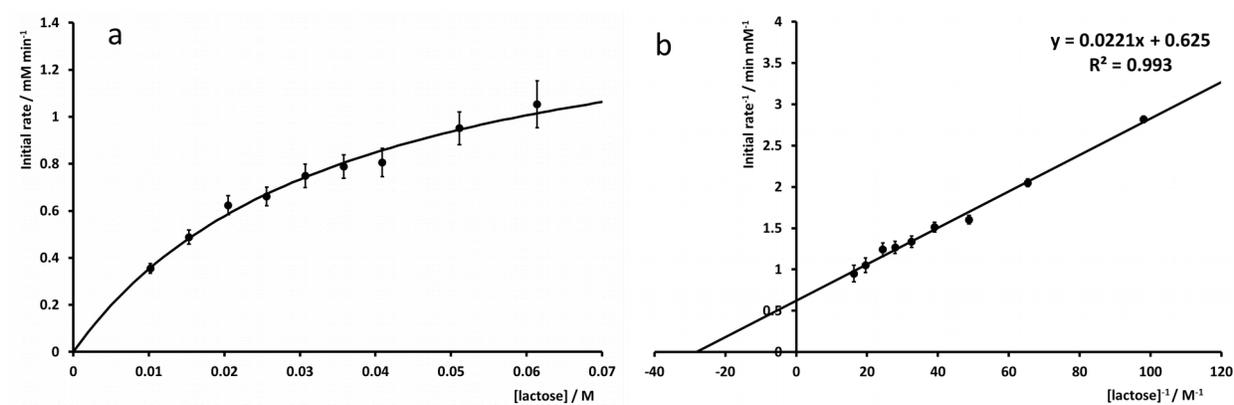
Figure II6: Rate of lactose hydrolysis (a) and Lineweaver-Burk plot (b) ( $T = 30^\circ\text{C}$ ,  $\text{pH } 5.0$ ).
