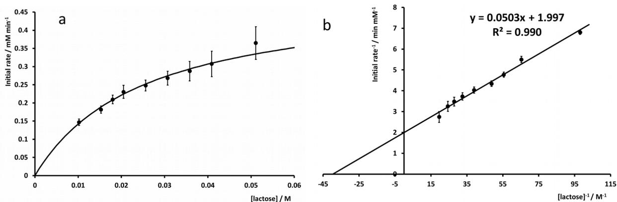
Figure II3: Rate of lactose hydrolysis (a) and Lineweaver-Burk plot (b) ( $T = 30^\circ\text{C}$ ,  $\text{pH } 5.0$ ).
