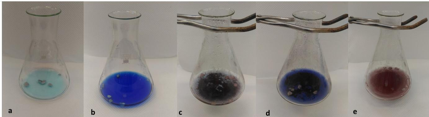
SH3: Steps of the titration: (a) Fehling A, (b) Fehling A + B, (c) Before indicator addition, (d) After indicator addition, (e) Endpoint.
