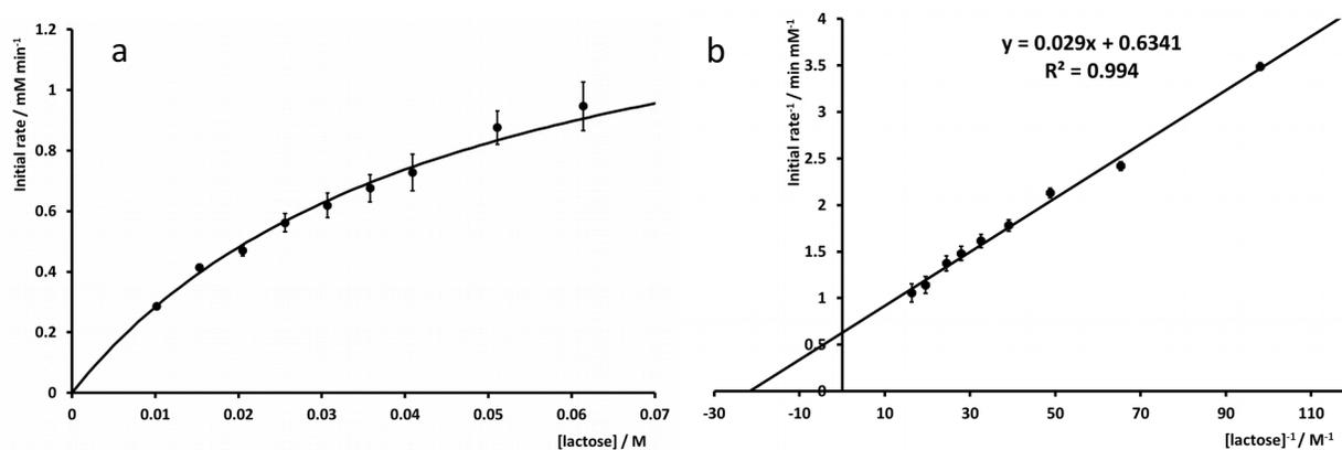
Figure II7: Rate of lactose hydrolysis (a) and Lineweaver-Burk plot (b) ( $T = 30^{\circ}\text{C}$ ,  $\text{pH } 5.0$ ).
